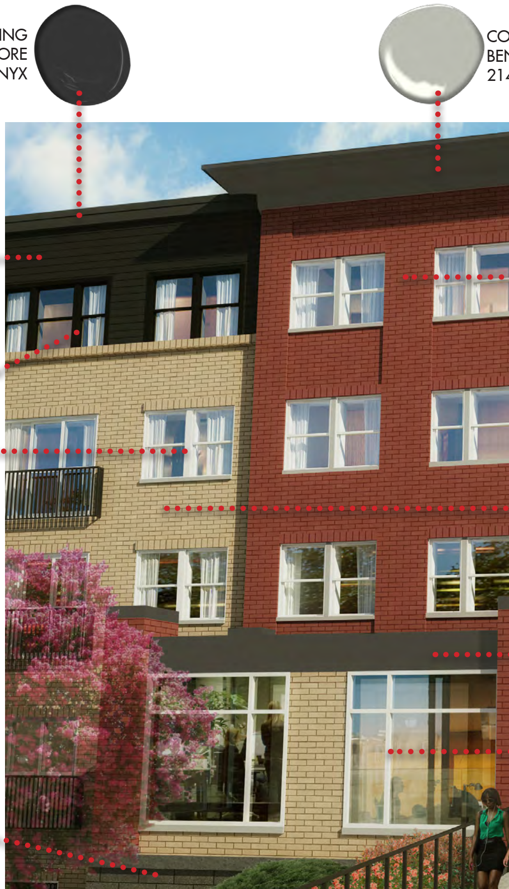
ACCENT BRICK VENEER CONTINENTAL BRICK - STANDARD #455 MOD. WITH SPECMIX "FIRESTONE" MORTAR
